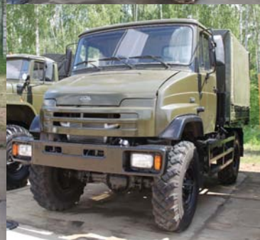
Left: the short wheelbase 4x4 ZiL-43272N has an all-terrain load capacity of 3000kg, a road speed of 90km/h and a range of 1000km.
