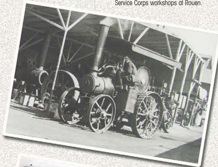
Below: this Fowler Tiger has just been rebuilt in the army Service Corps workshops at Rouen.
