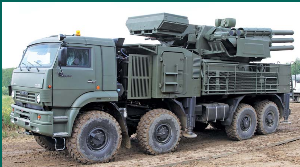
Above: the KamAZ-6560 is used as the chassis for the "Pantzyr-S1" SPADS.
