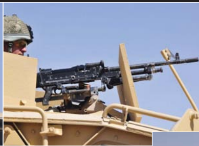
Left & far left: the Protected Weapon Stations fitted to the Utility Variant and the Command Variant of the Husky TSV-M feature perimeter protection as well as a gun shield.
