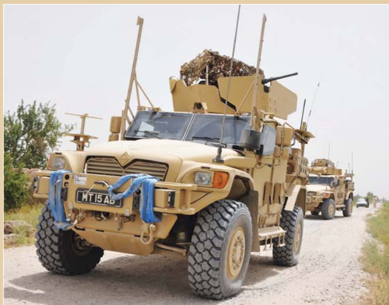
Left: compared to the Utility Variant and the Command Variant the Heavy Weapons Variant of the Husky TSV-M features a larger version of the Protected Weapon Station that can be fitted with a 7.62mm GPMG machine gun or a 12.7mm HMG or a 40mm L134A1 Grenade Machine Gun (GMG).
