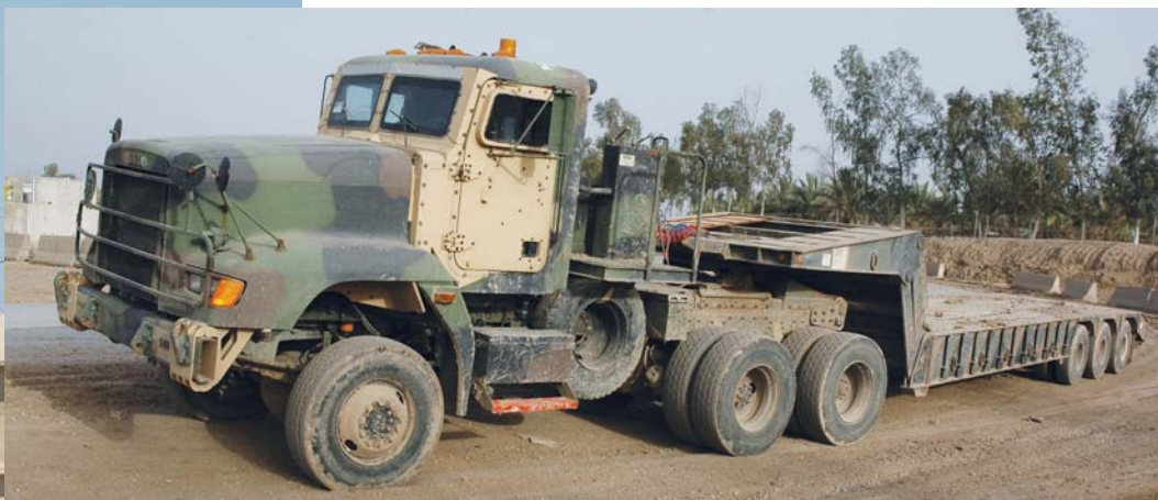
Left: in Iraq, a Freightliner-produced M916A2 and M870 40-ton lowbed trailer; note the easily identifiable cab armour package. (Carl Schulze)
